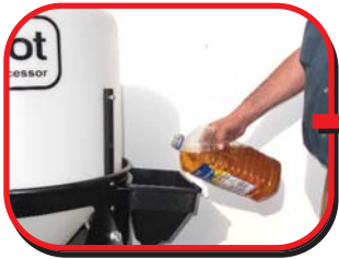
Add cooking oil to oil sump turn on heater (set to 60°C)
