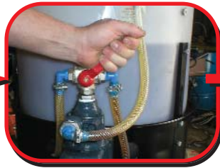
When oil is up to temperature, de-water using front sump valve. Set valve to 'Fill Vessel'
