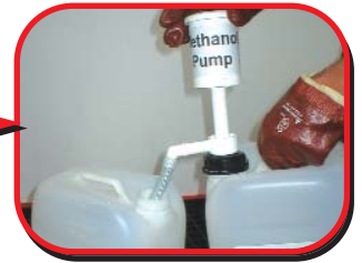
Mix methoxide in mix tank
