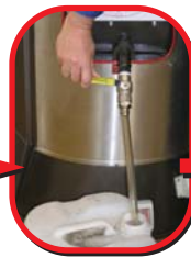
After 4-6 hours (or overnight) Drain glycerine from front tap
