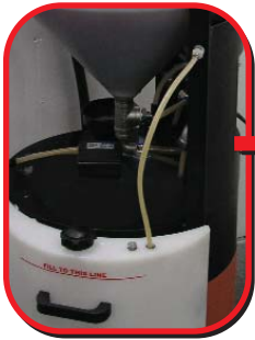
Connect mix tank to processor. Set front panel control to circulate (Add catalyst)
