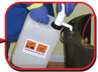
Mix methoxide in mix tank
