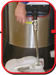
After 4-6 hours (or overnight) Drain glycerol from front tap
