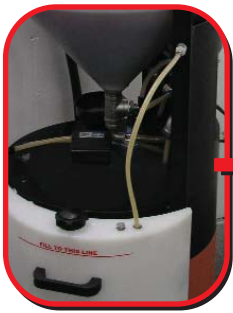
Connect mix tank to processor. Set control (Add catalyst)
