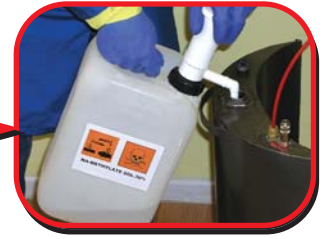
Mix methoxide in mix tank
