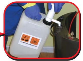
Mix methoxide in mix tank
