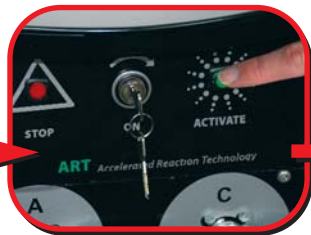
Activate ART system and drain off glycerine from front tap
