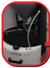
Connect mix tank to processor. Set front panel control to circulate (Add catalyst)
