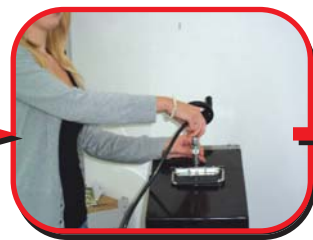
Water Wash Pump water filled vessel and connect to spray mister. Leave, drain off water. Repeat until clear. Re-heat Bio diesel to dry.
