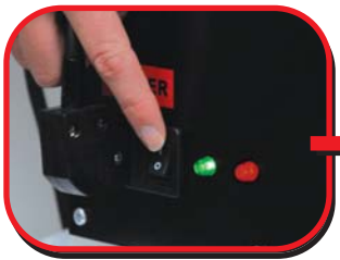
When Red light goes off, check oil temperature. Turn off heater.
