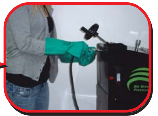
Agitate mix, while methoxide is being added.
