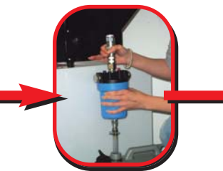
Dry Wash (optional) Connect dry wash tower. Open tap allow filtered bio to pass through.
